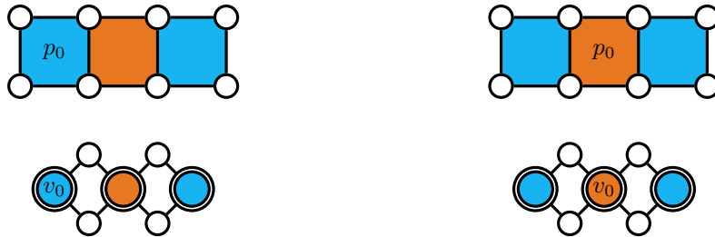
Figure 3.13: Two clusters of the same isomorphism class (first line) with their reduced König representation (second line). Structurally equivalent plaquettes within a cluster are given in the same color as well as bond vertices which are in the same or equivalent automorphism orbits of the reduced König representation. For this concrete example p_0 can be in the center (orange) or on one of the outer plaquettes (blue). On the structural level the outer plaquettes are indistinguishable, and the respective vertices of the reduced König representations are in equivalent orbits (blue).
