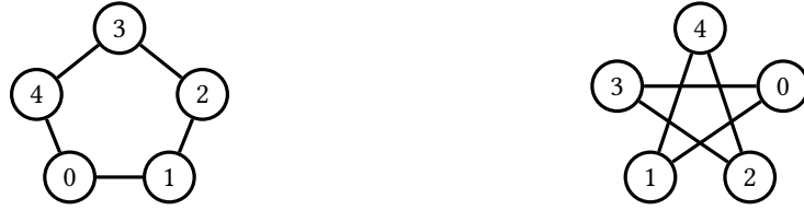
Figure 2.4: Two isomorphic graphs. An isomorphism from the left graph to the right graph is given by the mapping (0, 1, 4, 2, 3) . This example is also given in Ref. [157] with different names for the vertices.
