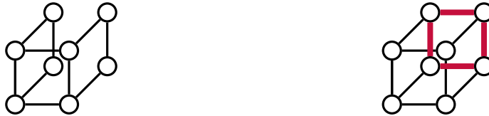
Figure 3.14: Adding a single plaquette to the cluster on the left, results in a cluster where any site is contained in an even number of bonds (right). The newly added plaquette is highlighted by thick red lines.
